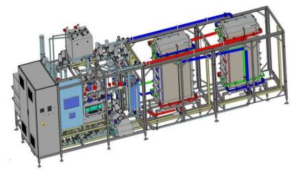
Technical Specification of Electrodialysis Equipment for Demineralization of Casein Whey^
